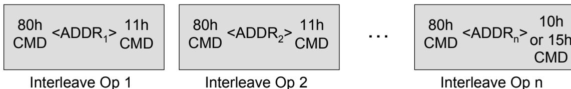
Figure 79 Interleaved Program (Cache)
