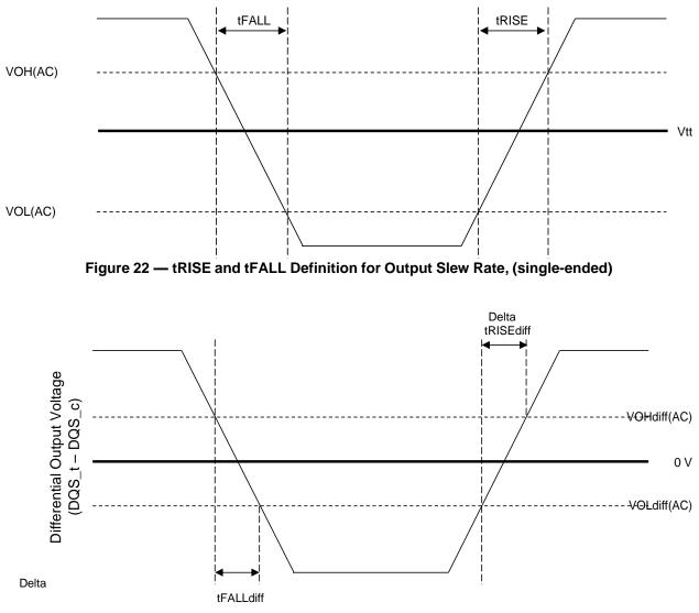
Figure 23 — tRISEdiff and tFALLdiff Definition for Output Slew Rate, (differential)
