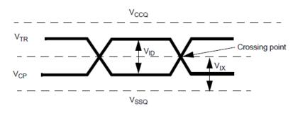
Figure 2 — Differential signal levels
